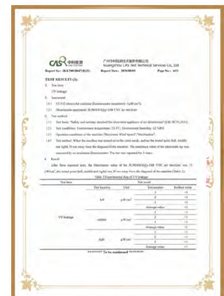
UV leakage test
