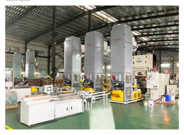
Guangdong-based Fortune Precision has launched a six-out conversion line for easy-open food ends, which is claimed to be the first in the world to manufacture 211-diameter steel easy-open ends for food cans.
