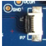
Figure 6 : Connection between DESPI-C03 and front light panel
