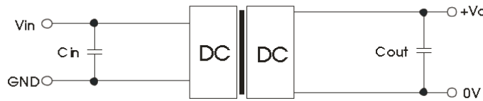
Note 1: Cin is 4.7uF/50V, Cout is 10uF/50V
